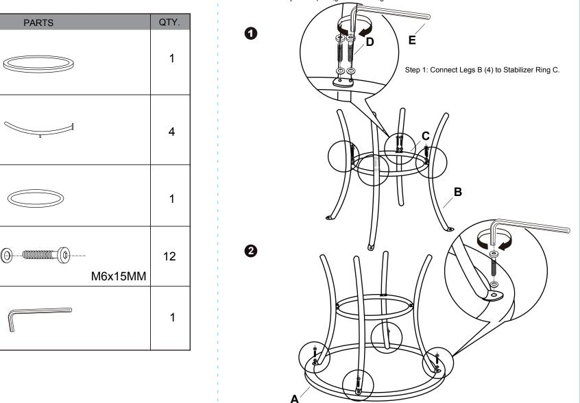
Step 2: Connect Leg and Ring Assembly to Tabletop A. Use care when laying table top on ground to avoid damage.
